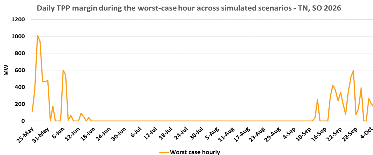
Figure 36 Minimum hourly TPP margin on each day of the analysed period in Tunisia.
