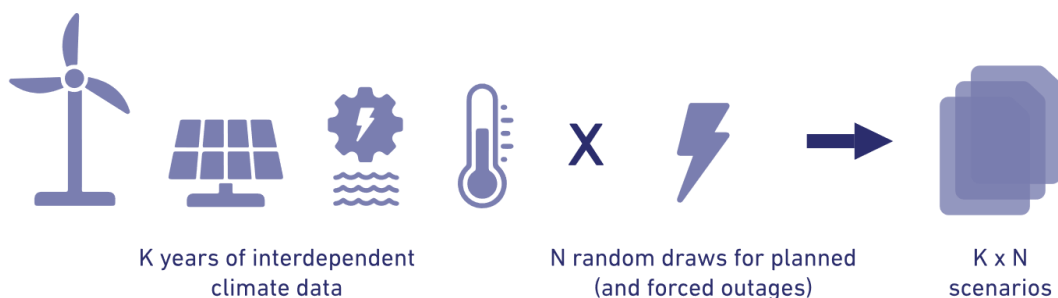
Figure 4 Probabilistic modelling general approach (source: ENTSO-E)
