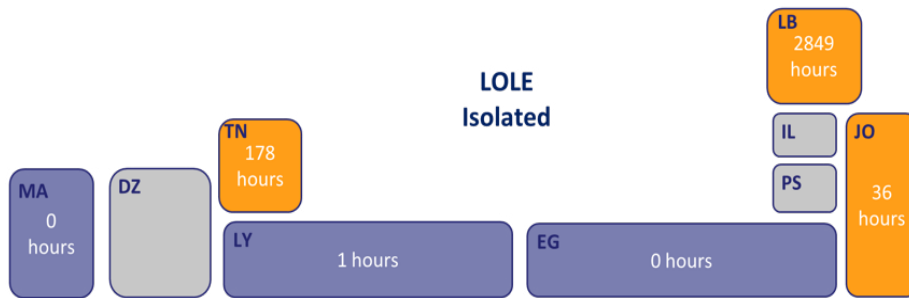
Figure 10 Seasonal relative EENS and LOLE for the isolated operational mode for the most severe MCY in summer.
